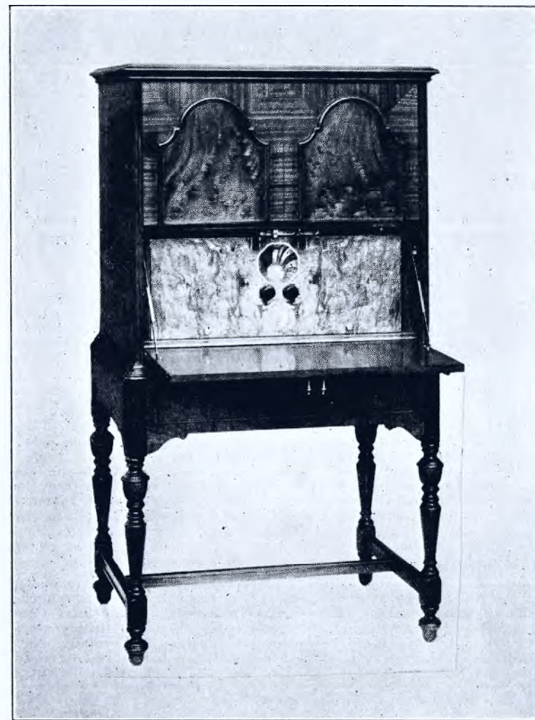
Fig. 3—Stromberg-Carlson No. 734-B Receiver. Drop Panel Open to show Location of Controls.
