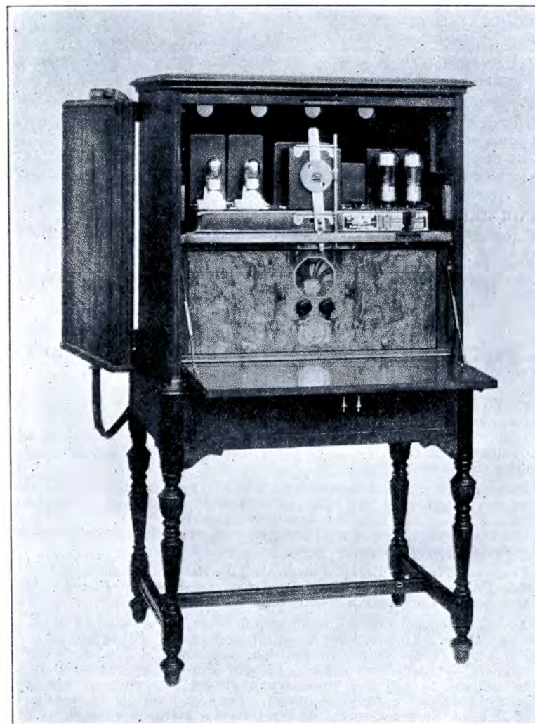
Fig. 4—No. 734-B Receiver, showing No. 404 Socket-Power Unit Installed in its Compartment.
