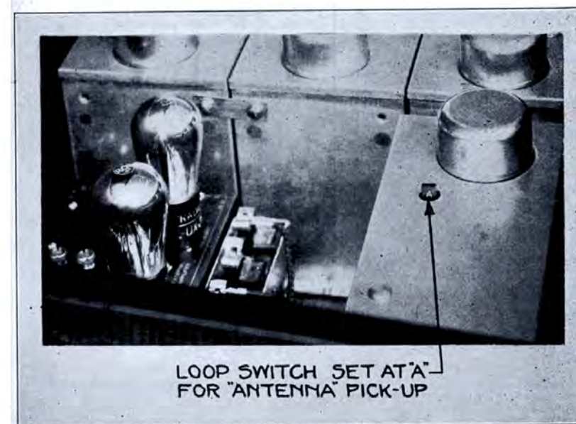
Fig. 50—Loop Switch in 1st Radio Shield, Set for Antenna Service "A"
