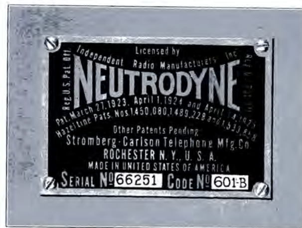
Fig. 52—License Plate attached to each Receiver Chassis, containing the Serial Number and Code Number of particular Receiver
