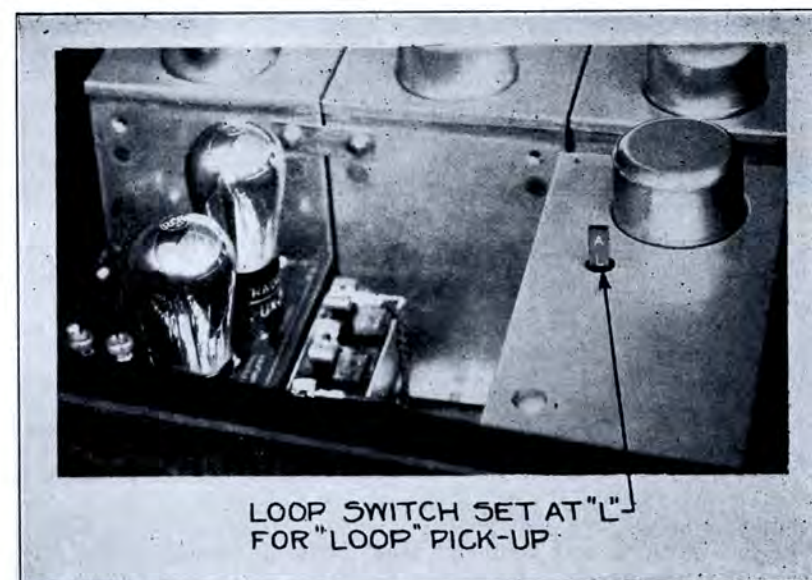
Fig. 49—Loop Switch in 1st Radio Shield, Set for Loop Service "L"
