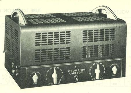
AMPLIFIER GROUND—A good building ground, such as a connection from a cold water pipe or the frame of a steel building, should be terminated under the knurled nut located on the rear of the amplifier.
